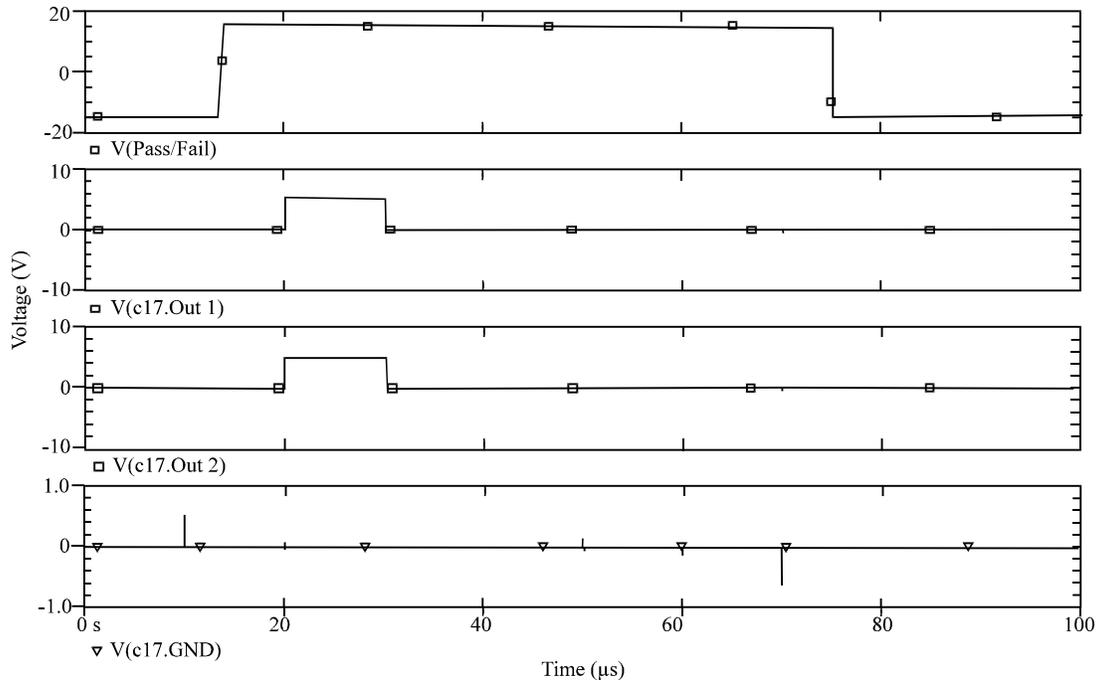
Fig. 8: Simulation Results of the Current Sensor with DUT Having Bridging Fault
