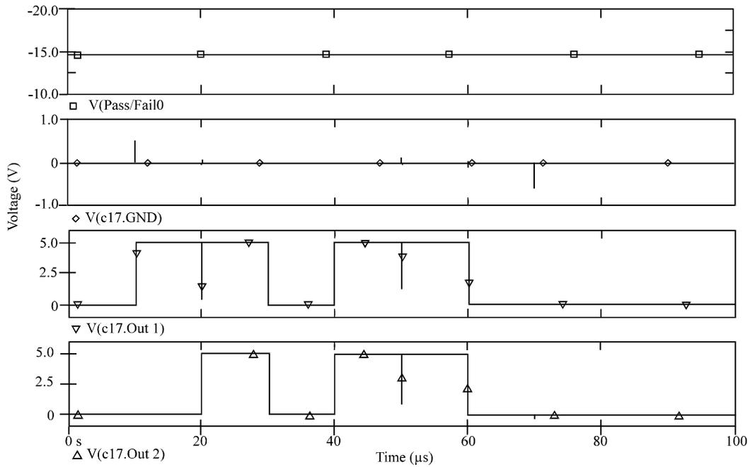
Fig. 5: Response of Fault-free DUT with Current Sensor
