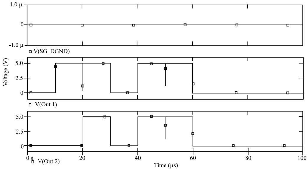
Fig. 4: Response of Fault-free DUT Without Current Sensor
