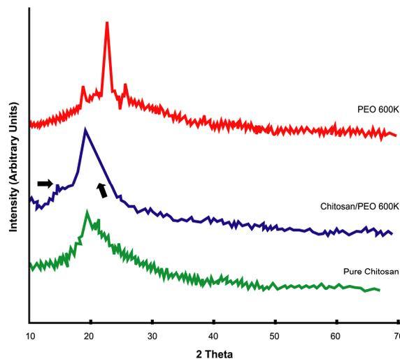
Fig. 7: X-ray diffractograms of pure PEO 600K, Chitosan-PEO 600K blend and pure Chitosan
