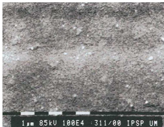
Fig. 2: SEM image of the pure chitosan membrane under 10,000 time's magnification
