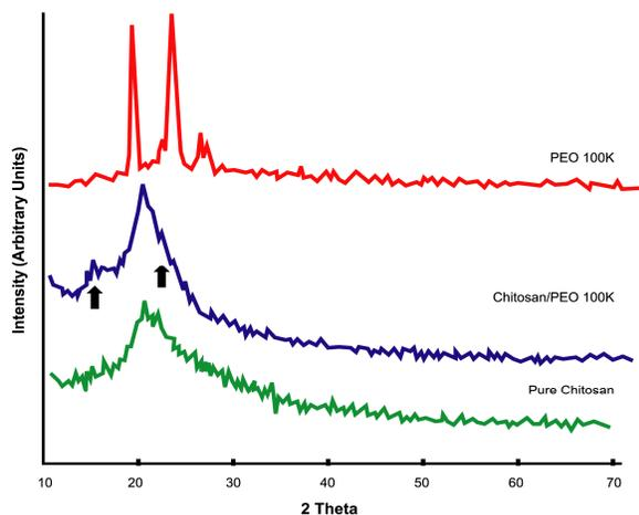
Fig. 8: X-ray diffractograms of pure PEO 100K, Chitosan-PEO 100K blend and pure Chitosan
