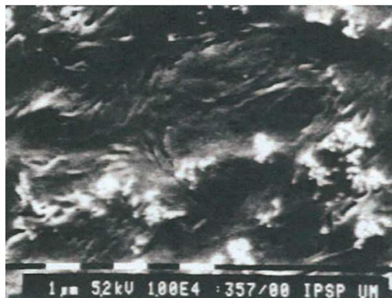
Fig. 3: SEM image of the pure PEO 600K membrane
