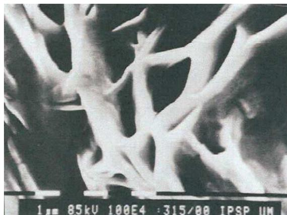
Fig. 4: SEM image of the pure PEO 100K membrane
