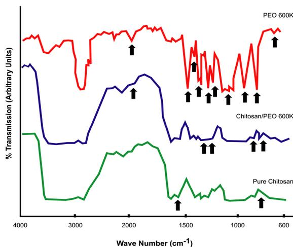
Fig. 9: IR spectra for PEO 600K, Chitosan-PEO 600K blend and pure Chitosan
