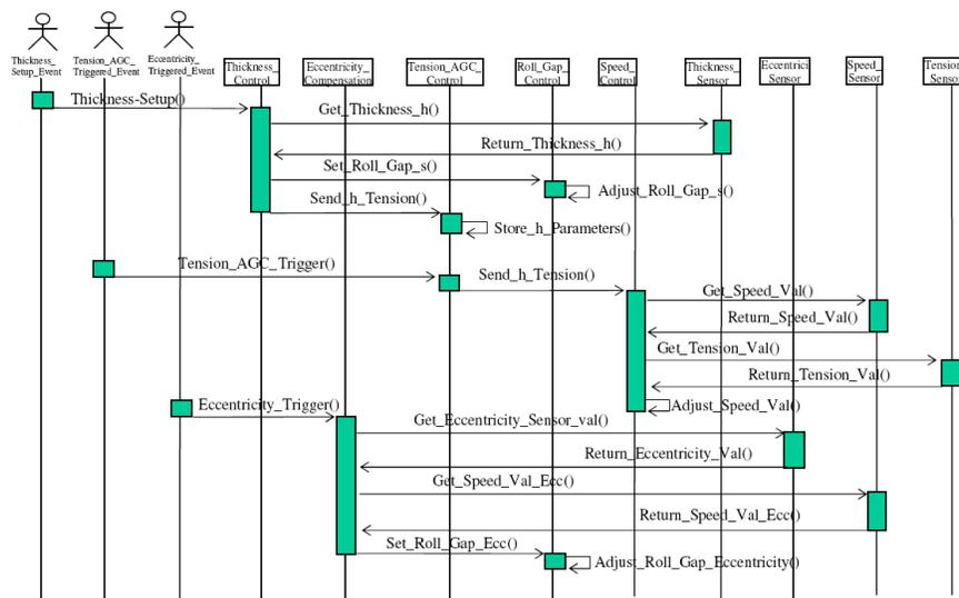
Fig. 3: Sequence Diagram of Automatic Gauge Control System
