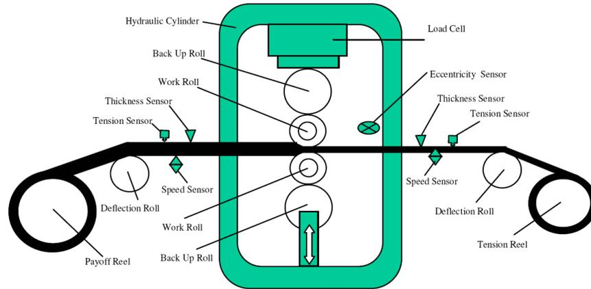
Fig. 1: The Reverse Rolling Mill
