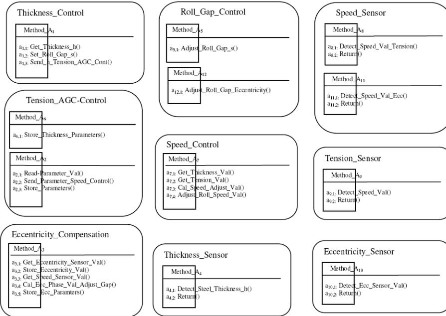
Fig. 4: Method Description of Automatic Gauge Control System
