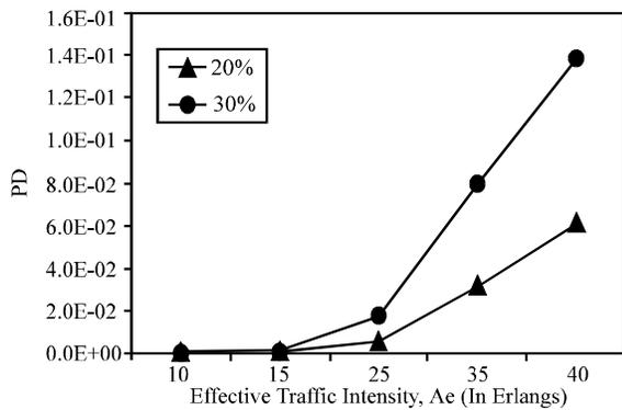
Fig. 1: Probability of Delay versus Effective Traffic Intensity for Different Outage Load where  $N=100$  and  $\gamma=0.00664$
