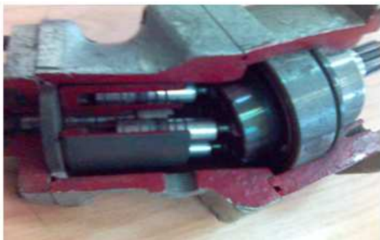
Fig. 8. Spatial mechanical transmission, ball, the cylinders and the pistons, used to pumps and motors rotating
