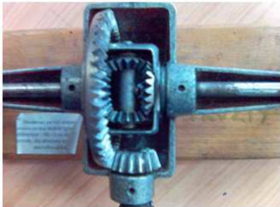
Fig. 6. A differential mechanism
