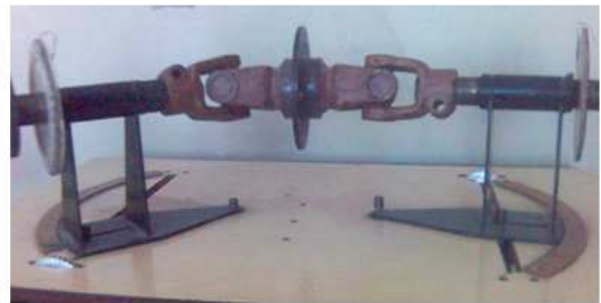
Fig. 4. A mechanism with an universal joint and the other one with two universal joints and the mini shaft
