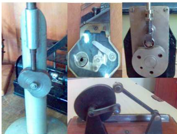
Fig. 3. Mechanisms with rotary cam and follower
