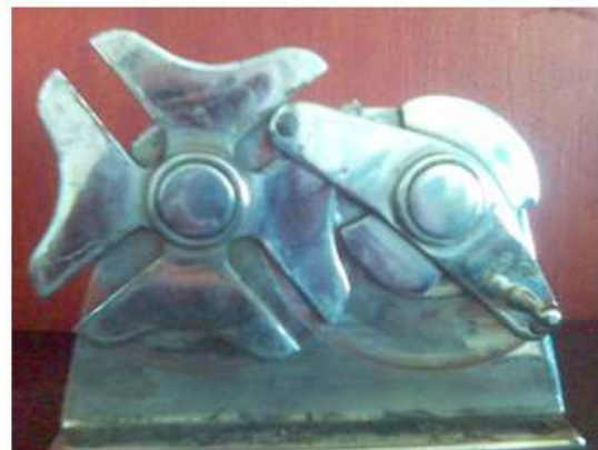
Fig. 5. A Geneva drive mechanism (Mechanism with cross of Malta), first one with one beginning and second one with two beginnings
