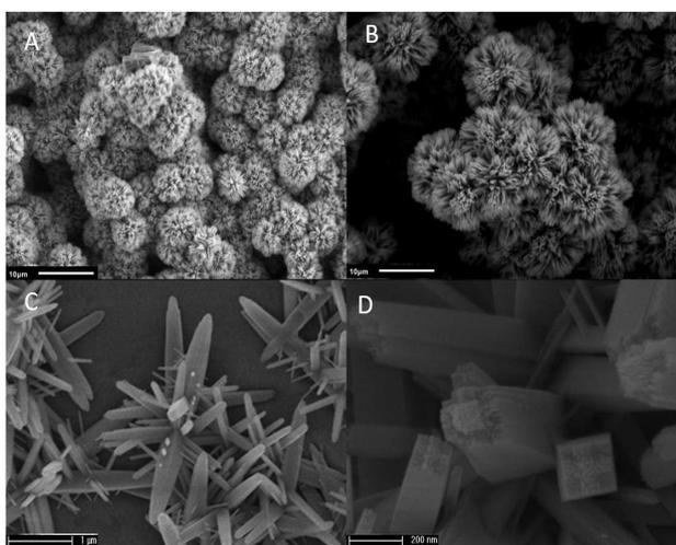
Fig. 2. SEM images of the as-synthesized TiO<sub>2</sub> NWs at different magnifications: 2,500x (A); 5,000x (B); 33,000x (C); and 50,000x (D)
