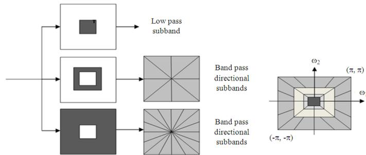
**Fig. 1.** Nonsampled contourlet transform (a) Nonsampled filter bank structure that implements the NSCT (b) Idealized frequency partitioning
