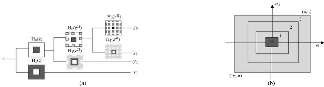
**Fig. 2.** Nonsampled pyramid (a) Three-stage pyramid decomposition. (b) Sub bands on the 2-D frequency plane
