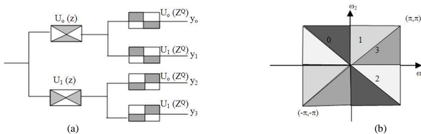
**Fig. 3.** Four-channel Nonsampled directional filter bank constructed with two-channel fan filter banks. (a) Filtering structure (b) Corresponding frequency decomposition
