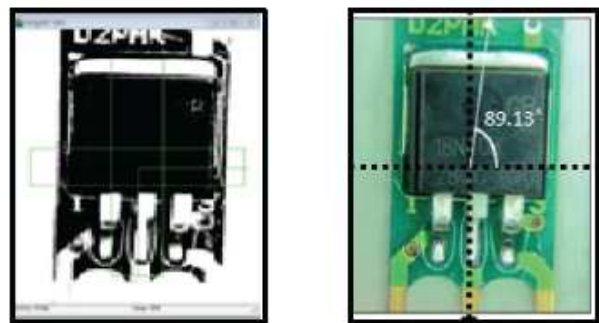
Fig. 5. The rotated image (with flux defect) and image Converted to 8-bit unsigned grayscale
