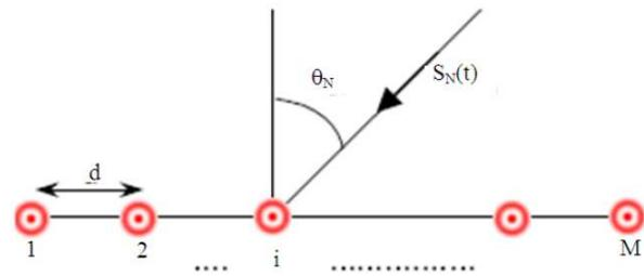
**Fig. 1.** Uniform linear array antenna configuration
