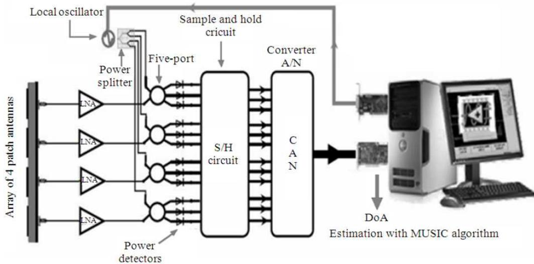
Fig. 3. Complete schematic of the DOA estimation system
