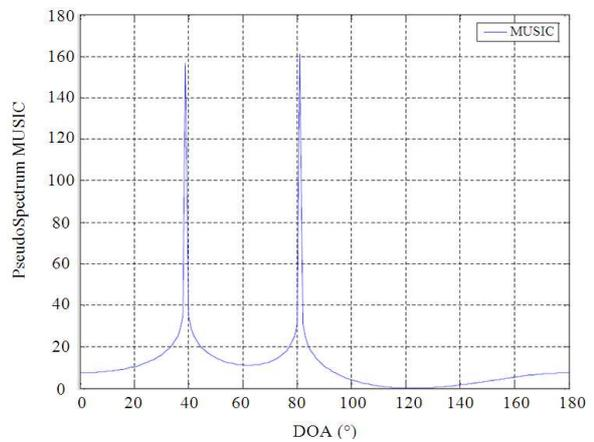
Fig. 4. Simulation result of three uncorrelated signals at the DOA of 40°, 80° and 90° with 100 snapshots
