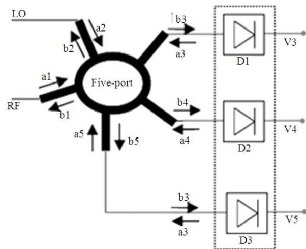
**Fig. 2.** Five-port circuit with three diode power detectors
