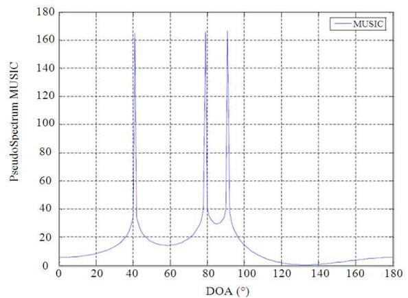
Fig. 5. Simulation result of three uncorrelated signals at the DOA of 40, 80 and 90° with 200 snapshots
