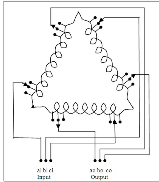
Fig. 3: Delta connected tapped autotransformer
