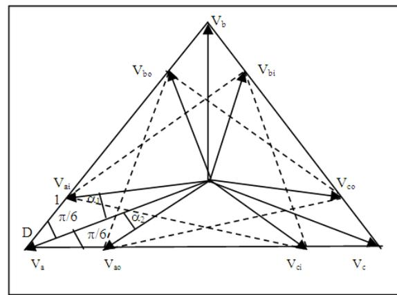
Fig. 4: No-load phasor diagram
